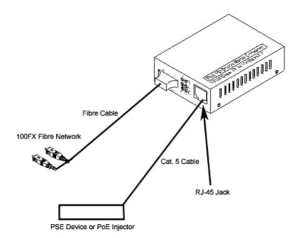
Fig. 2 Example connection between POE120, PSE device and Fibre Cable
