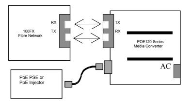
Fig. 3 POE120 Series to PSE Device or POE Injector
