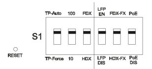
Fig. 11 Reset button and S1 – Bit 1, 2, 3, 4, 5, 6, Configuration and Settings
